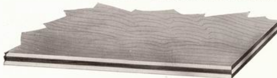
Section showing Triple-Veneer Bottom
