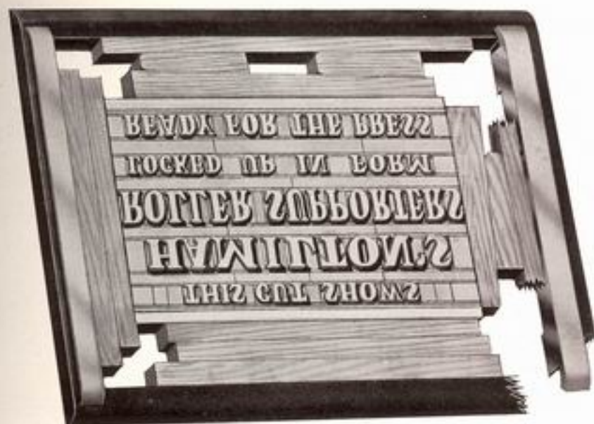
A Pair of Roller Supporters Locked in Job Chase
