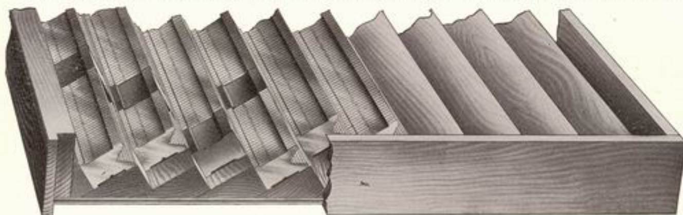
Detailed Section of Matrix Drawer, showing Matrices in place with Letter Stamp facing the front
