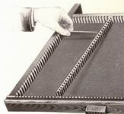
Showing Method of Subdividing a Drawer to fit Electros and Cuts
