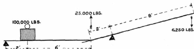
If it takes 25,000 lbs. of energy to raise 100,000 lbs. Weight (see illustration above) placed two feet from the end of an eight foot lever, by the addition of another lever ten feet long with a fulcrum two feet from its end it takes only 6,250 lbs. (friction added) to do the same work.
