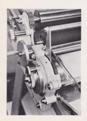
The cylinder height is adjusted with a calibrated drum to provide any height from under type high to 5 points over.
