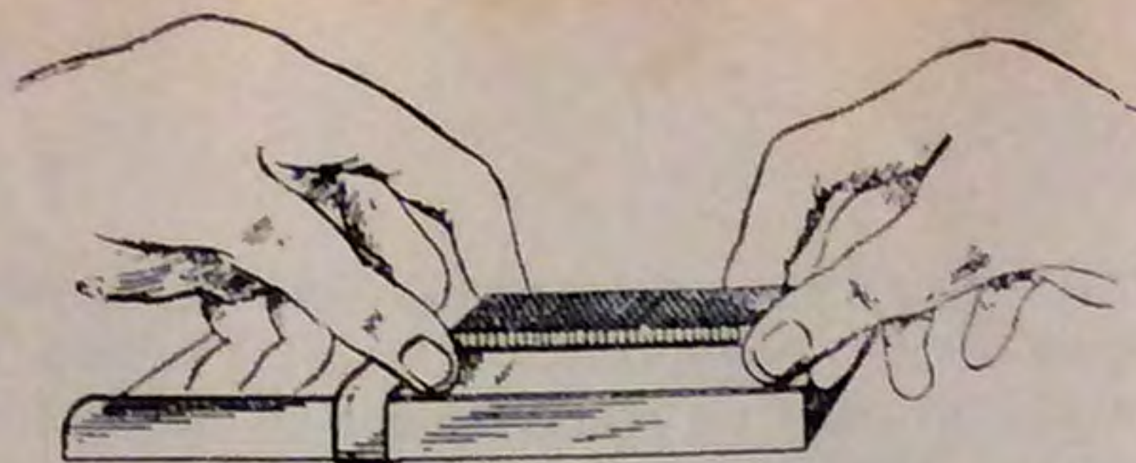
Fig. 11. Removing a "stickful" of type from the composing stick.
